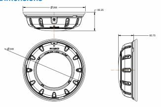
Waterco's Litestream LED Replacement Kit comes with a twistlock adapter plate that can easily replace a majority of surface mount pool lights.
