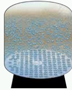
Uniform introduction of air and water through the nozzle plate provides vigorous agitation and filter media bed expansion required for an effective air/water backwash leading to reduced backwashing times and reduced volumes of water.
