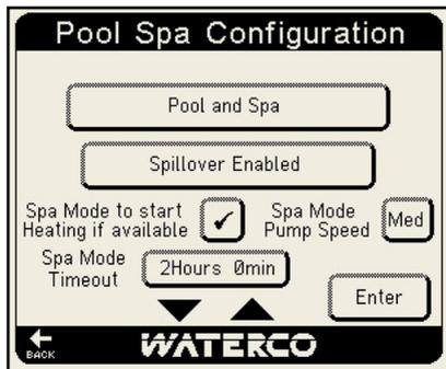
If heating is to start when SPA MODE is selected ensure the check box is ticked and Spa Mode Timeout is programmed and press Enter to the next screen.
