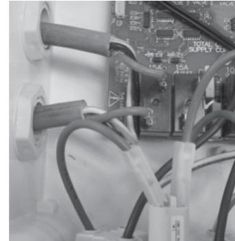
The Aquamaster features 2 x 15amp dry contact switching relays which may be used to operate equipment with an electrical rating of up to 15amps each. Ideally, a separate electrical supply with circuit breaker protection should be connected to each 15amp switching relay numbered 6 & 7 on the PCB.
