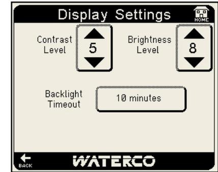
The user may adjust screen settings of Contrast Level and Brightness Level by selecting the relevant icon up and down arrows to the desired display setting. The backlight timeout may also be adjusted by pressing the relevant icon until the desired timeout is selected.
