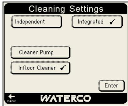
If the installed system is fitted with a Cleaner Pump select the “Cleaner Pump” icon and press “Enter”.
