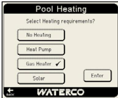
If “Gas Heater” or “Heat Pump” is selected the “Gas Heater Settings” or Heat Pump Settings” Menu will appear.
