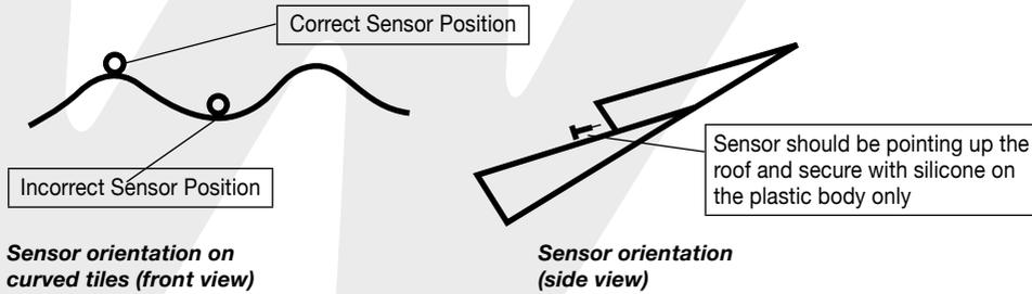
The sensor should be orientated such that it lies on the crest of the roof tiles and not in the troughs. This eliminates water being trapped in the silicon glue that holds the sensor in place, and giving erroneous readings. The roof sensor should also be positioned so that it points up the roof tiles (as shown above).
