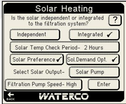
Press the “Solar Temp Check Period” icon to alter the period between the system checking the pool temperature via operation of the filter pump. The period may be set to check between one and four hours in half hour increments.
