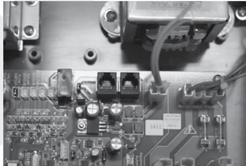
Each touch screen control is to be wired to the Aquamaster Control Box. The maximum cable length from the touch screen control to the Aquamaster Control Box is 50 meters. Recommended minimum cable size is 24AWG (7/020) or Category 5 shielded data cable.
