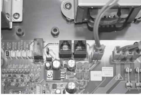
The Aquamaster system comes complete with one touch screen control. An additional screen available separately may be connected providing additional operational convenience to the owner. There is a small jumper link on the circuit board which must be removed.
