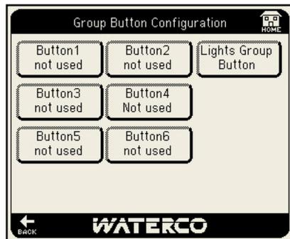
To program a group button press any icon showing “not used”. On the next screen press the icon “Edit Group Button” which allows the programmer to select from installed equipment a pre programmed sequence of multiple functions operated from one named icon.
