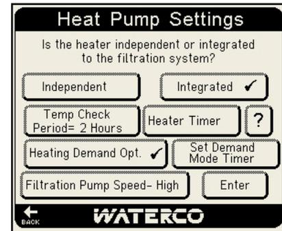
Press the “Temp Check Period” icon to alter the period between the system checking the pool temperature via operation of the filter pump. The period may be set to check between 1 and four hours in half hour increments.
