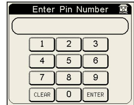
The Aquamaster default PIN code is 1234 > Enter. To change the PIN enter the “Change User PIN” screen through the Configuration Menu. Enter the new PIN > Enter and then Confirm New PIN by re entering the same PIN number again > Enter.
