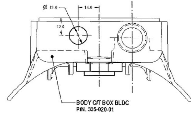
Step 4 – When the hole is drilled remove the locking nut from the cable gland and thread the cable through the hole so that the plug is now located within the motor control box. Thread the lock nut over the cable and screw onto the cable gland and tighten.
