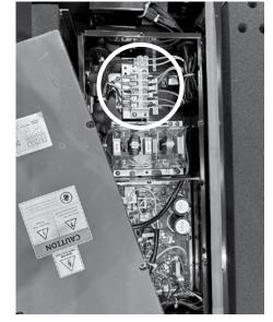
Remove terminal box lid and locate P1 & P2 for connecting the pump control relay and terminal 5 & 6 for connecting external automation heater control.
