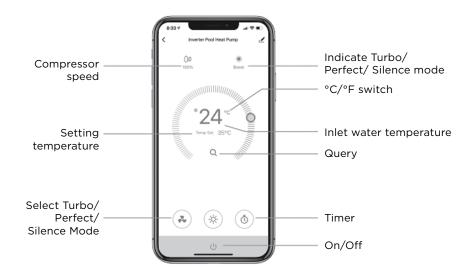
2. For heat pump with Heating & Cooling function:
