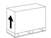
The heat pump is supplied mounted to a pallet. Once transported to site, remove the screws securing the pallet to the unit to install on the prepared slab / brackets.
