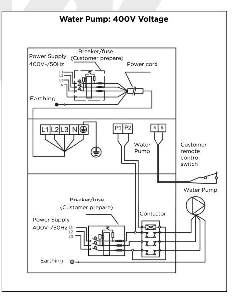
**Note:** Do NOT connect the water pump directly to P1 & P2.
