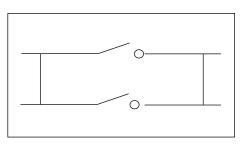
2: Water pump wiring of Heat Pump
