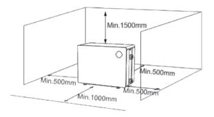
Figure 1. Manufacturers installation clearance guidelines
