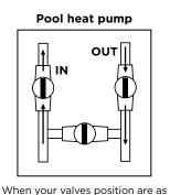
When your valves position are as shown on Figure 1, the water is bypassing the pool heat pump.
