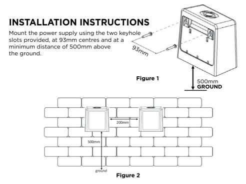
The LED Pool Light transformer to be mounted at minimum of 500mm above ground level. Multiple units should be mounted at minimum of 200mm from each Transformer and a minimum distance of 500mm from any other electrical equipment or device. Electrical Terminal Connections should be on underside of unit. Refer Figure 1 & 2.
