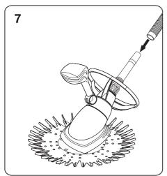
Connect sufficient lengths of cleaner hose to cover the distance from the pool skimmer box to the furthest point of your pool, plus one length.
