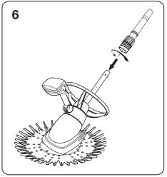
Slide the outer tube assembly down the inner tube and screw the hand nut into place as this will secure the deflector wheel.
