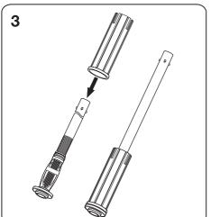
Place the diaphragm cartridge over the top of the cleaner inner tube with the larger opening to the diaphragm and retaining ring and slide down the inner tube and ensure the retaining ring is properly secured into the cartridge. Note: Ensure the diaphragm is not twisted once installed into diaphragm cartridge.
