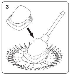
Place the cleaner shroud (Silver) over the inner tube and slide down onto the main body. The main body has a location key that needs to align with a groove within the shroud. This ensures the shroud is installed correctly.
