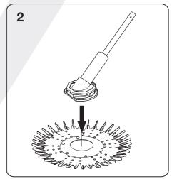
Place the inner lip of the fined disc onto the flexi foot pad flange and peel over until disc is secure between the flange and lip of the flexi foot pad. The fins of the disc and the word "TOP" should face the cleaner main body.
