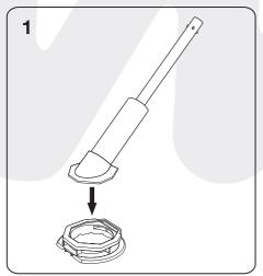
Fit flexi foot pad to cleaner main body ensuring the main body lower flange is properly secured into the flexi foot locating groove.
