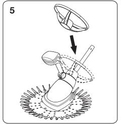
Slide the cleaner deflector wheel over the inner tube until located on top of the float assembly. The deflector wheel does not align with the locating key on the main body and is able to spin freely on the top section of the main body.
