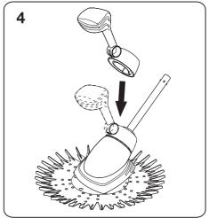
Place the cleaner float assembly over the inner tube and on top of the shroud. This also needs to be aligned to the main body location key.
