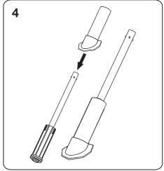
Insert the diaphragm, retaining ring and inner tube assembly into the main body and ensure the diaphragm cartridge is pushed fully into main body. The diaphragm is assembled ready for the remaining Swimkleen 2 components to be assembled.
