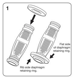
Place Diaphragm retaining ring over one end of the Swimkleen 2 diaphragm. Ensure the retaining ring is properly secured into the locating groove of the diaphragm.
